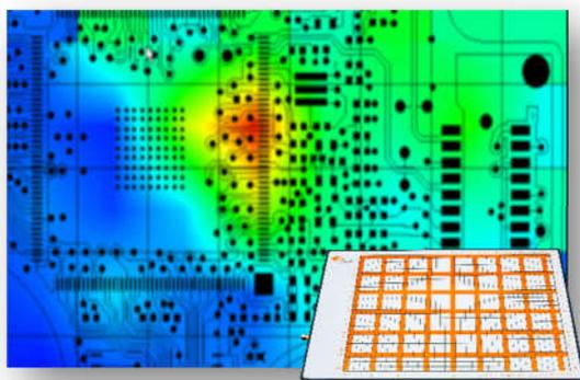
EMC and signal integrity are major concerns in the design of ultra-high speed (>2 GHz) PCBs. EMSscanner enables the design engineers to diagnose EMC/EMI problems between 150 kHz and 8 GHz.
